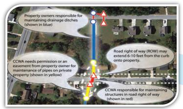
The diagram above shows the level of service provided by CCWA's Stormwater Utility. Everything shaded in yellow is maintained by the utility.
